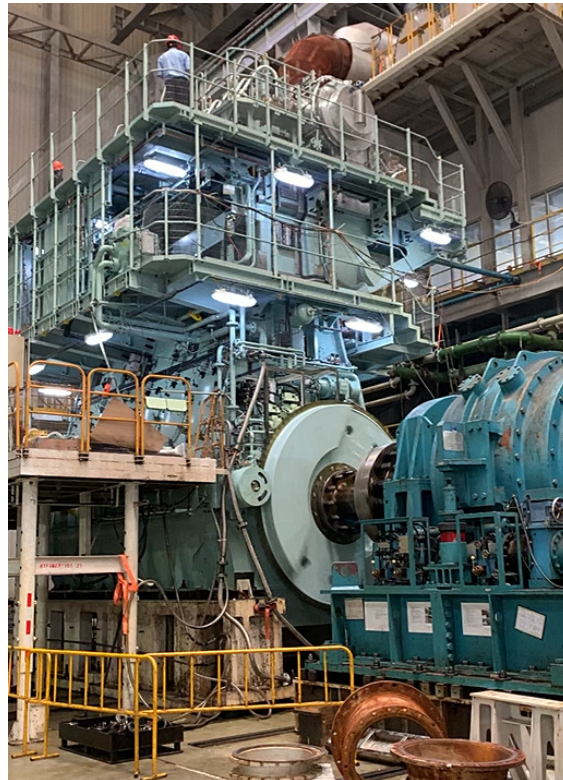
Engine undergoing a factory acceptance test on one of YCMP's test stands.
