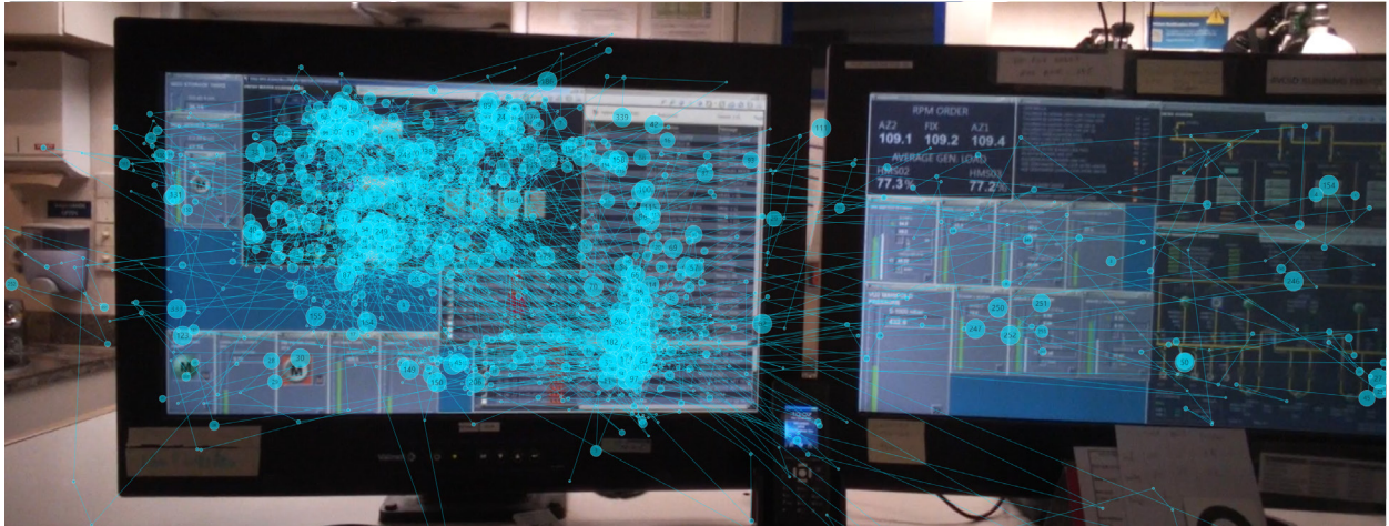
Figure 22. Dynamic gaze trajectory mappings with fixation lengths between 300ms (smallest circles) and +1000ms (largest circles) on the alarm list HMI on a large passenger ship.
