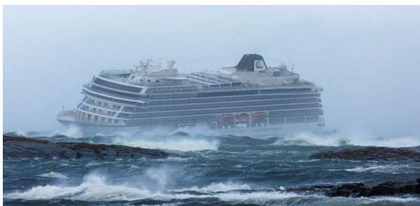
Figure 1. Viking Sky in a near-grounding vicinity to shallow banks [6, p. 98]. The auxiliary engines' automatic shutdown due to low lubrication oil pressure caused the ship to drift ashore, as it lacked power for its electrical propulsion.
