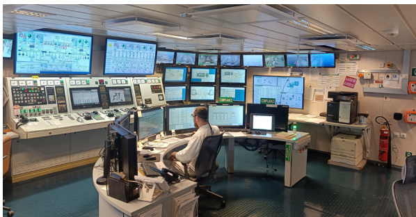
Figure 4. Watchkeeping engineer in the ECR on a passenger ship carrying more than 8000 people.
