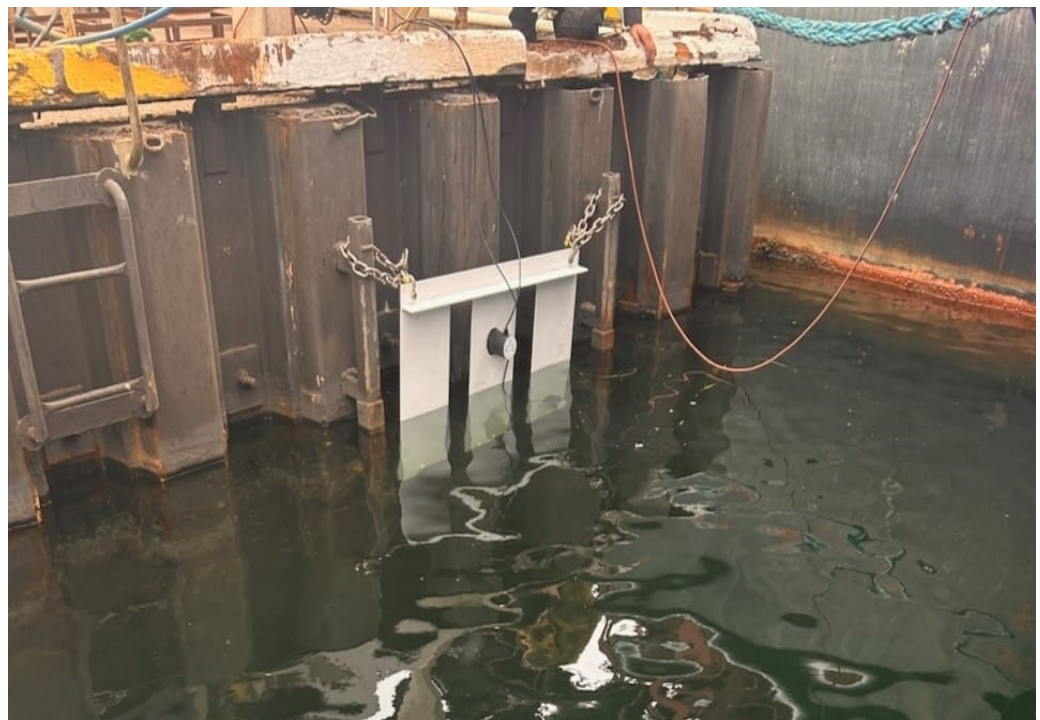
Figure 2.7 Test panels with ultrasonic transducers, one above and one below the water surface, in the Sea Harvest Yard, South Fremantle.
