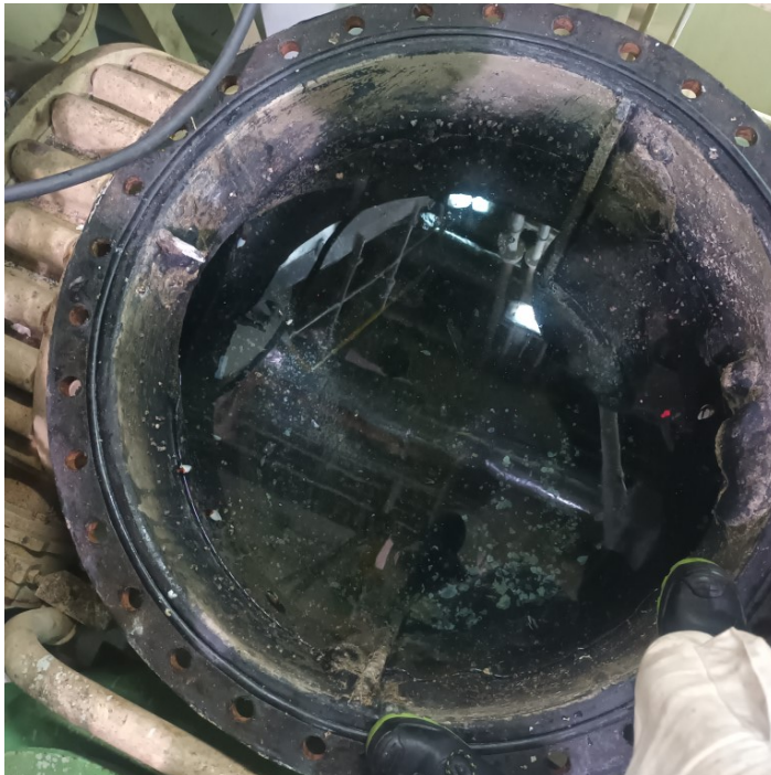
Figure 3.1 High sea chest strainer found without marine growth, i.e., fouling rating 0, when opened on 16 th April 2025.
