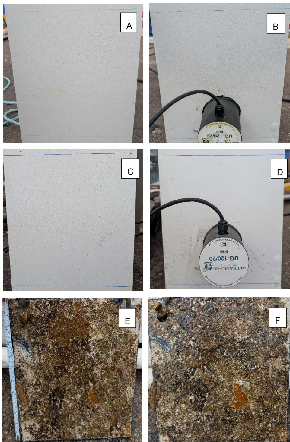
Figure 3.6 Test and control panels submerged in water in South Fremantle, Western Australia. Test panels were found without fouling after 55 days (A and B) and 69 days (C and D). Control panel was found with heavy macrofouling meeting fouling rating 4 after 55 days (E) and 69 days (F). The ultrasonic transducers were mounted on the test panels above the water surface (A and C) and below the water surface (B and D).
