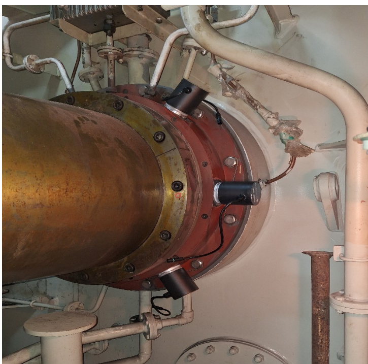
Figure 2.2 Ultrasonic transducer installed on top of pipe leading to low-temperature (LT) cooler No. 1.
