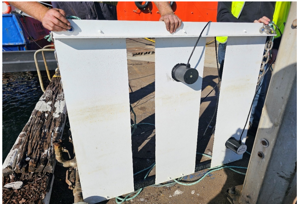
Figure 2.6 Ultrasonic transducers glued on test panels.
