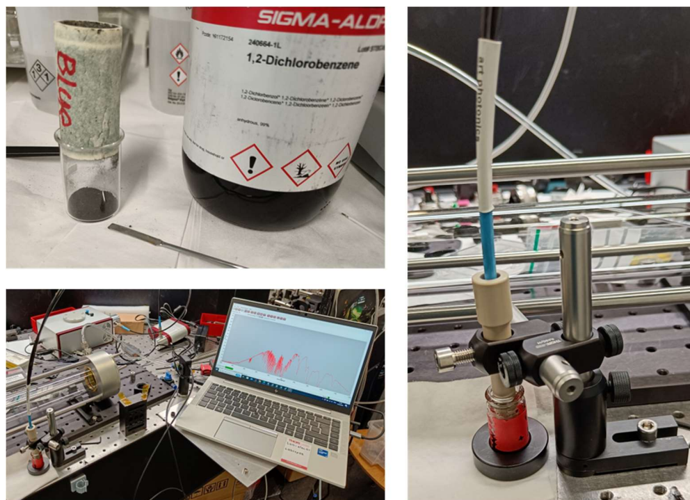
Figure 18. Photographs from the particle analysis using ATR-FTIR spectroscopy. (Top, left) Extraction of dust from the particle filter before subsequent mixing with a solvent. (Right) ATR probe submerged into slurry of dust and solvent. (Bottom, left) Setup and raw spectrum recorded.
