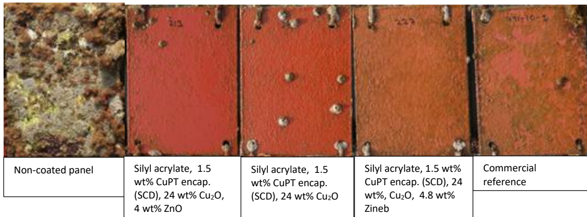
Figure 12. Coatings with a Silyl acrylate binder system and Encapsulated CuPT Super critically dried (SCD), and Cu 2 O after 6 months of static sea exposure
