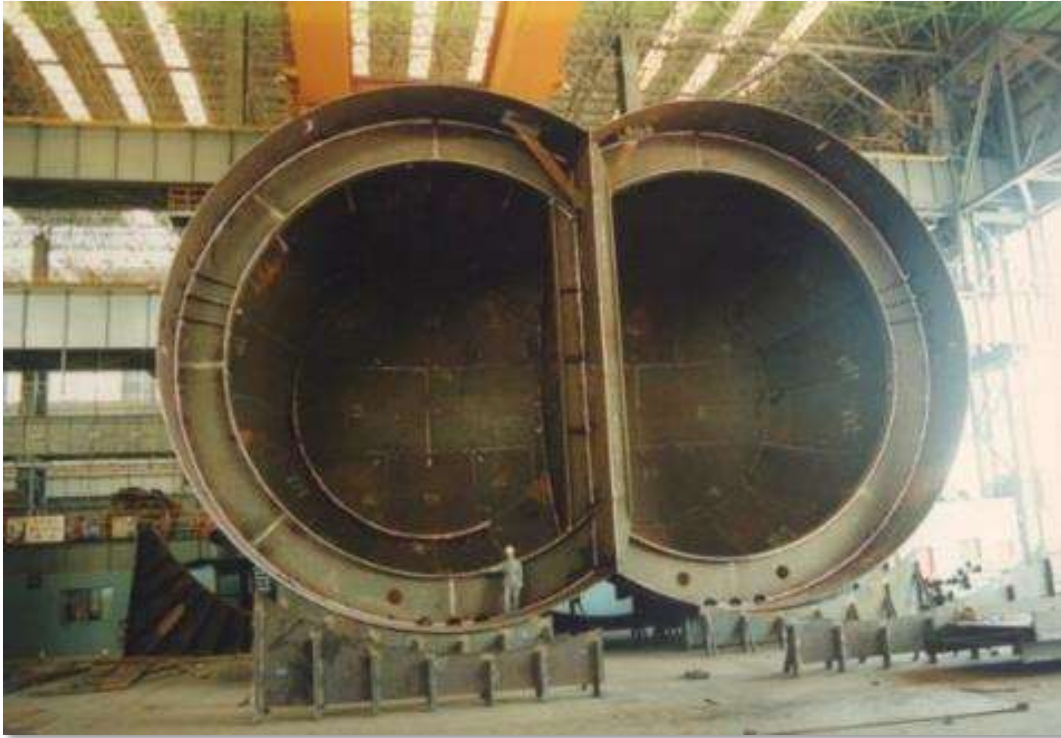
Fig 6 Bi-lope cargo tank type C
