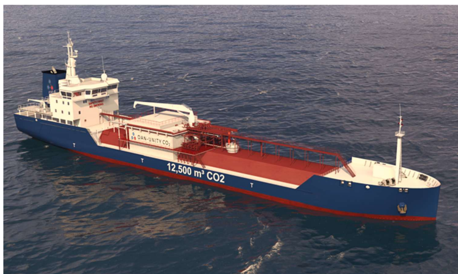
Fig 40 12,500 m 3 LP CO 2 carrier
