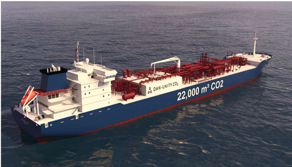
Fig 43 22,000 m 3 LP CO 2 carrier
