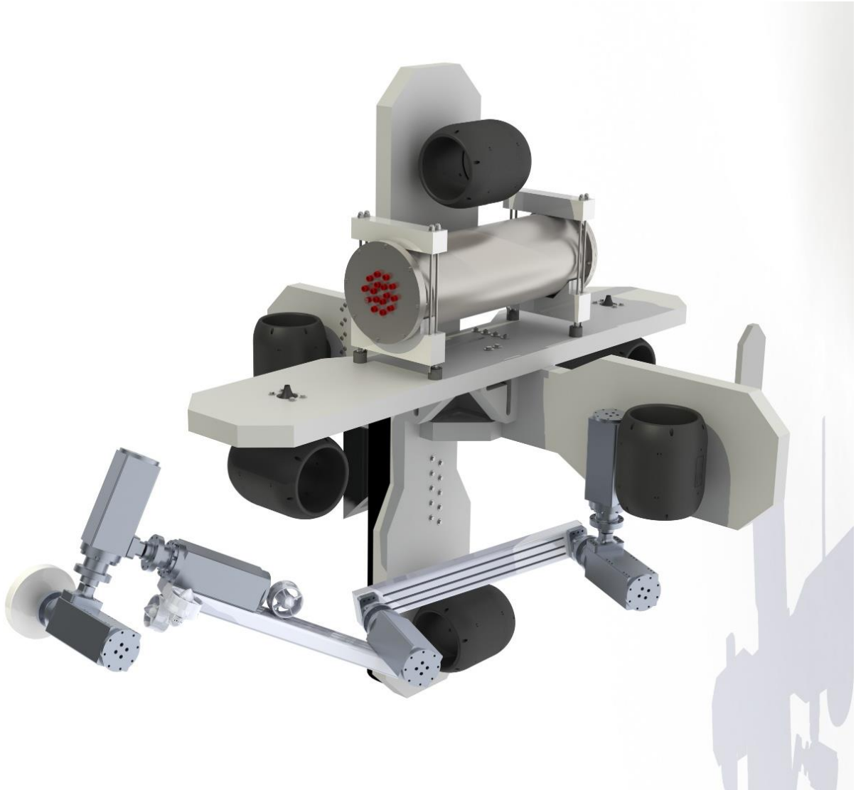
Figure 1 3D computer model of ROV, with robot arm attached
