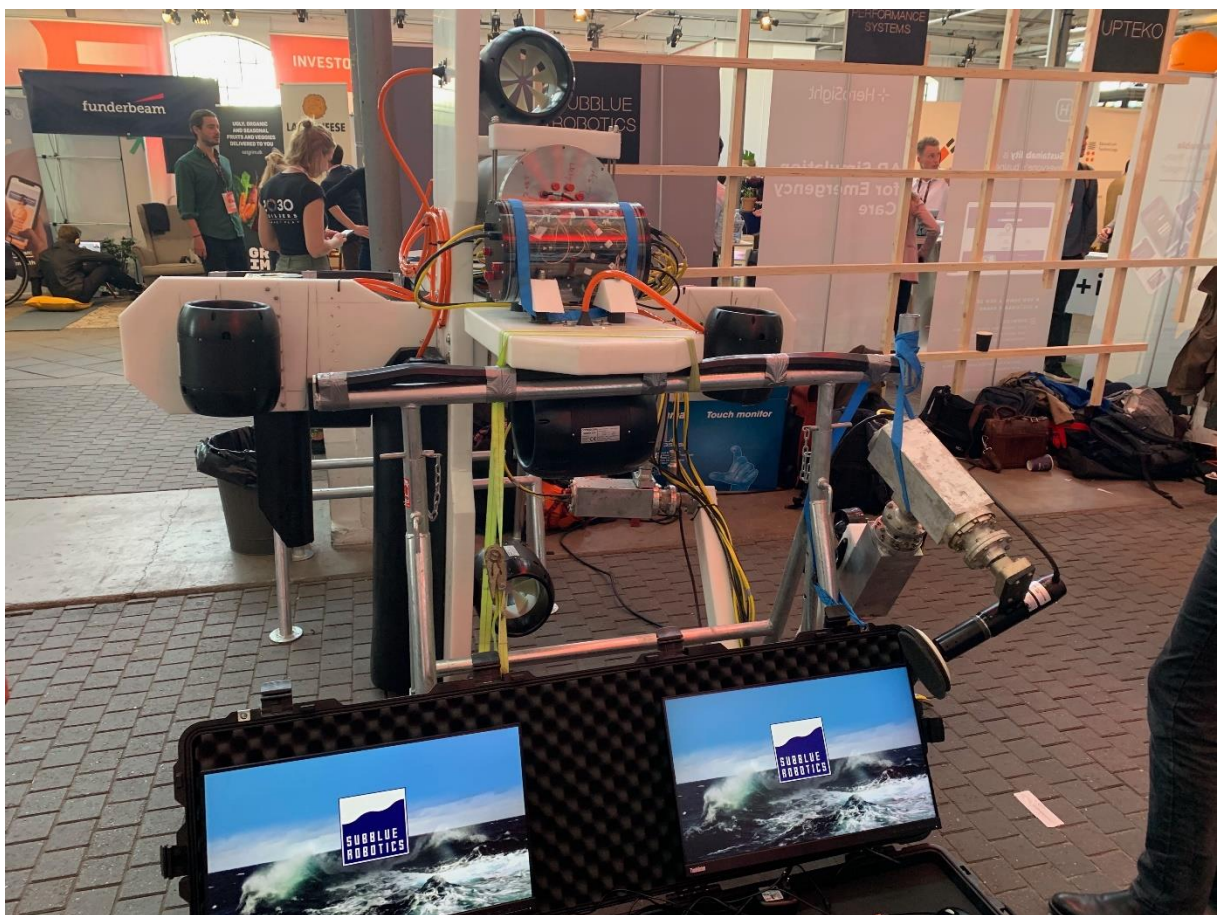
Figure 4 Robot arm and ROV combined
