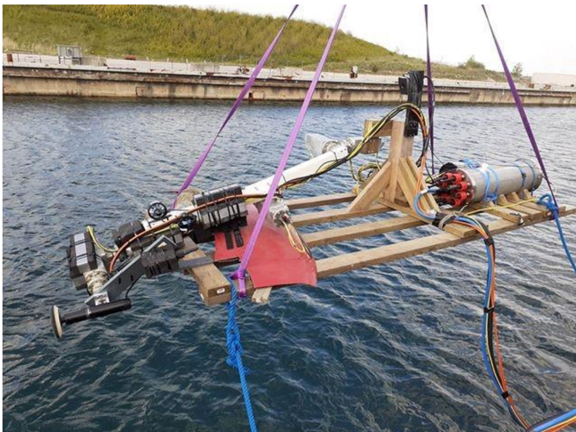
Figure 8 Robot arm on submersible test-rig with test-surface for polishing
