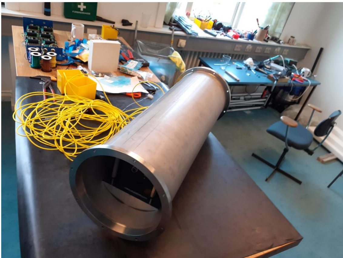
Figure 22 Submersible tube for holding electronics
