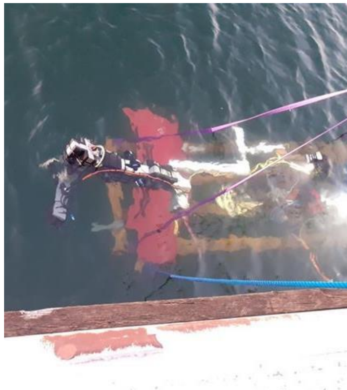
Figure 7 Robot arm on test-rig in harbor, while maneuvering to polish a test-surface
