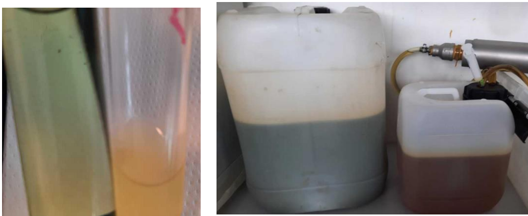
Figure 9.: Long term 1 month exposure of MGO to Lagur system showing clear oxidation effects of the EMF treatment, reference MGO remained unchanged. Left picture: a 5 ml sample of ref MGO (green tube) and 1 month exposure (yellow tube), Right picture: the two cans with reference MGO (left large can) and 1 month exposed MGO (right small can).
