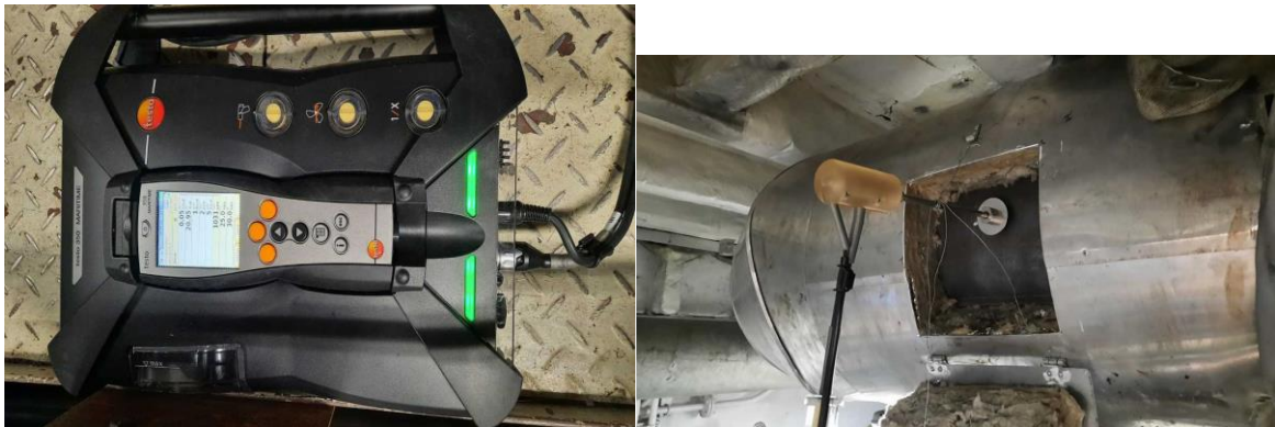
Figure 16: Left: TESTO 350 gas analyzer sensor box, Right: Gas Probe inserted in the center of the engine exhaust pipe.
