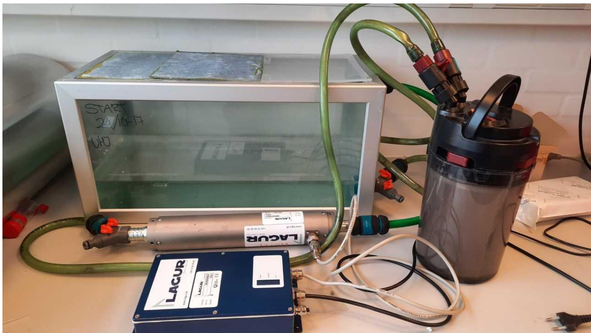
Figure 19: The continuous flow system for testing of EMF on water
