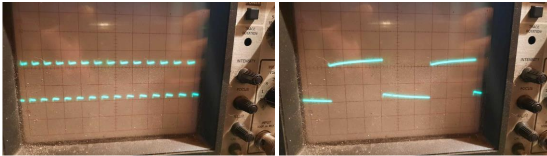
Figure 3: Two distinct signal patterns measured directly from the internal electrical signal to the coil. Signal is 10 volt peak to peak and 1 to 5 Ampere pulsed with varying with at 1 to 5 KHz period.
